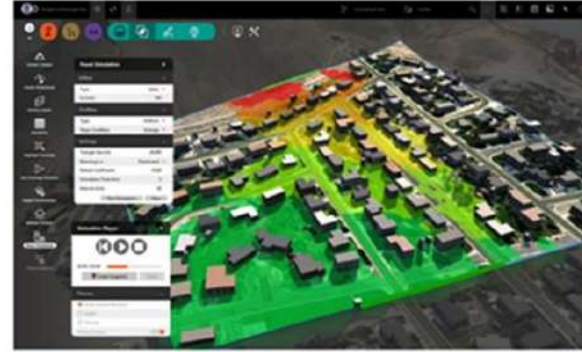
BIM SOFTWARE CAN BE USED TO SIMULATE THE FLOODING CAUSED BY ADVERSE WEATHER, IDENTIFYING HIGH RISK AREAS.
